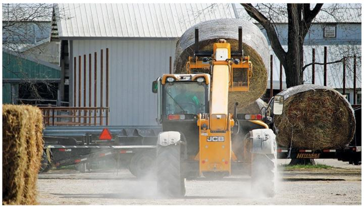
An enclosed operator compartment and an attachment designed to hold bales improve bale handling safety.
