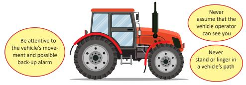
Blind spots are typically located directly behind or in front of the vehicle and in front of the rear wheels.
