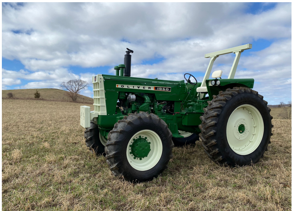
Tractor retrofitted with ROPS, courtesy of Iowa farmer, Easton Halverson
