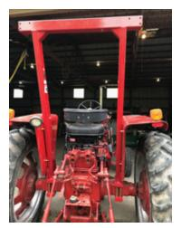
A 1971 International 656 tractor before and after a ROPS was installed
